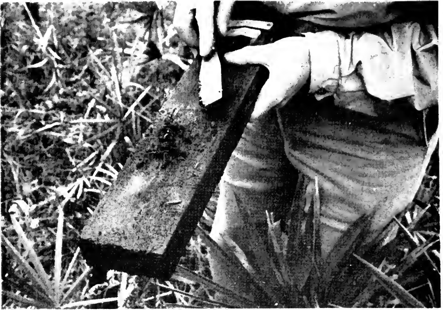
Fig. 1 (a)—Oak specimen treated with chromated zinc arsenate, showing surface softness due to decay.
